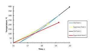
Fig. 3. Comparison of Temperature in Experiments and FEA at the Same Point.
