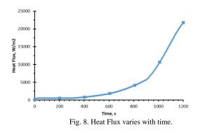
After observing the next step we analyze the magnitude of heat flux on glass sheets that have been simulated on Mecway FEA, obtained in Fig. 7 and .8 the magnitude of indexed heat fluxes Radiant heat from the front of the glass side exits through the back side of the glass with a minimum heat flux of  $20.94 \text{ kW} / \text{m}^2$  in 1198 seconds equal to 19.97 minutes and maximum heat flux of  $21.69 \text{ kW} / \text{m}^2$ .
