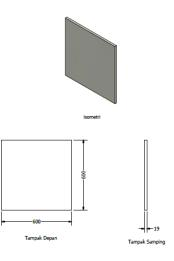
Fig 2. The Dimension of float glass
