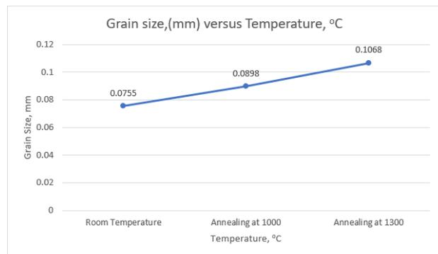
Figure 5: Line graph grain size, mm versus temperature, °C
