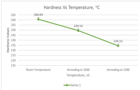
Figure 3: Hardness values versus temperatures.
