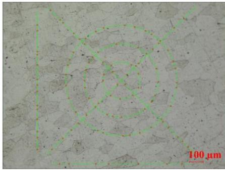
Figure 4: Grain size analysis for sample at room temperature.
