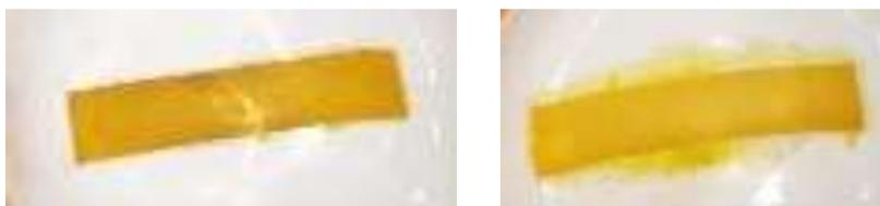
Figure 2 . Observation after Prototype Test-Strip Impregnated with Iron (III) Chloride Reagents dropped with Extracted Sample show visually yellow or bright yellow if paracetamol absence
