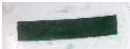
Figure 3 . Observation after Prototype Test-Strip Impregnated with Folin Ciocalteu Reagents dropped with Extracted Sample show visually dark green if paracetamol presence
