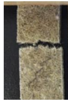
Figure 8. Experimental crack propagation trajectory done by Hao [12]
