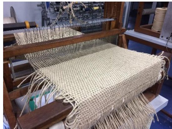
Figure 1. Weaving of kenaf yarns using table loom
