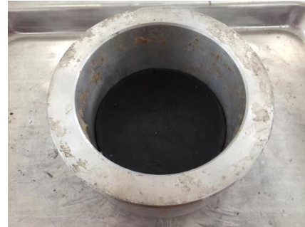
Figure 2. Mixture poured into mold cavity
