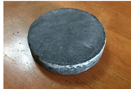
Figure 3. Rice husk silica specimen
