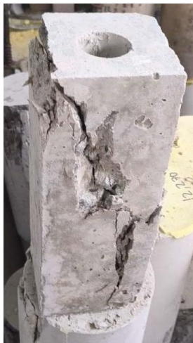
Figure 13. Prism Concrete Without Pipe Hole Variation 1 ¼ inch Shear Crack Type
