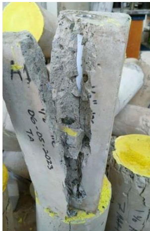
Figure 8. Prism Concrete With 1/2 Inch Hole Variation Pipe Columnar Crack Type
