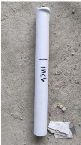
Figure 4. 1 Inch Diameter PVC Pipe Test Results
