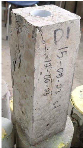
Figure 12. Prism Concrete With 1 ¼ inch Hole Variation Pipe Columnar Crack Type
