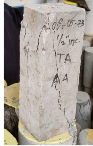
Figure 9. Prism Concrete Without Pipe 1/2 inch Hole Variation Columnar Crack Type
