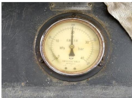
Figure 3. The pressure gauge found on the Hydraulic Jack-In Pile machine Source: Documentation, 2023
