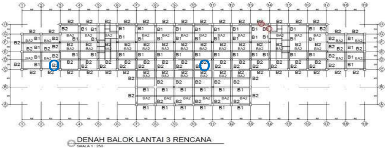
Figure 3.8 Hammer Test Points for Beams and Plates
