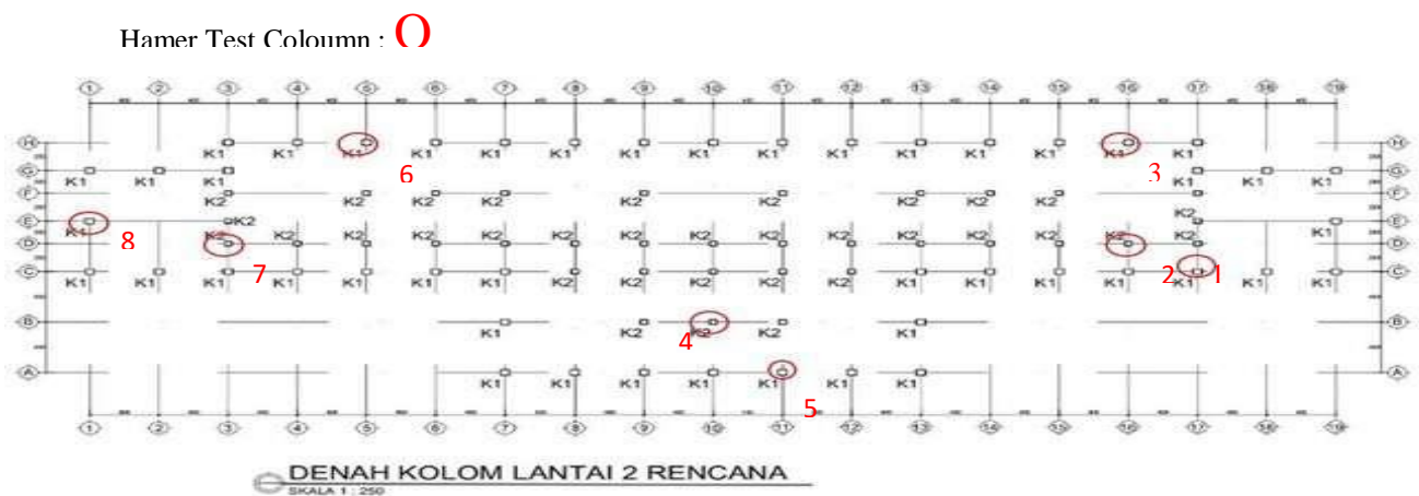
Figure 3.7 Column Hammer Test Point
