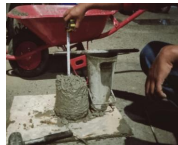
Picture 7. Slump Test (Source : Personal documentation, 2023)
