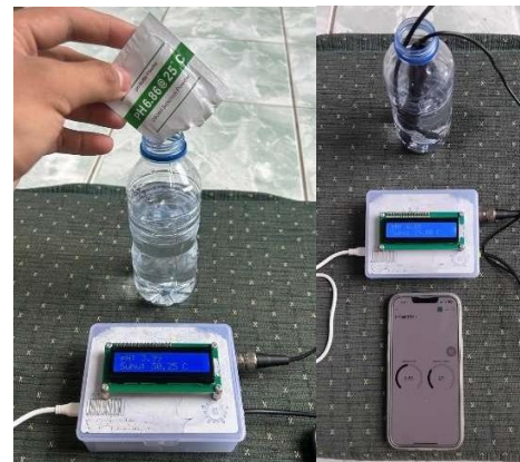
Figure 15 Calibration results with pH meter powder with a pH level of 6.86
