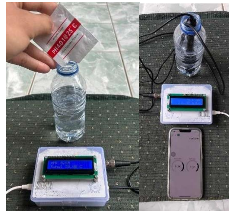
Figure 14 Calibration results with pH meter powder with a pH level of 4.00
