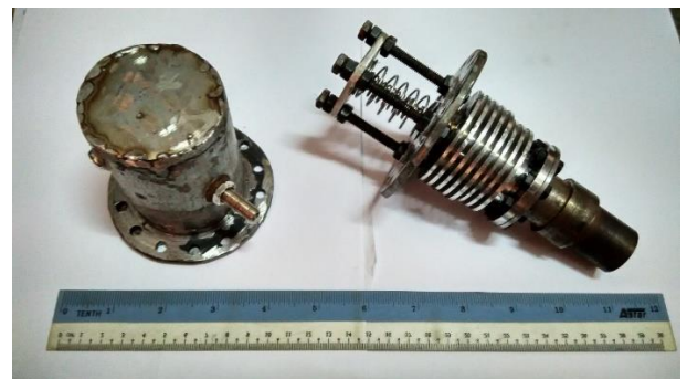
Figure-13: The fully assembled free piston Stirling engine prototype and its top cover.
