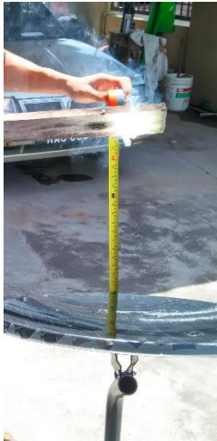
Figure-19: Focal length measured from the bottom edge of the parabolic dish (approximately 500 mm).
