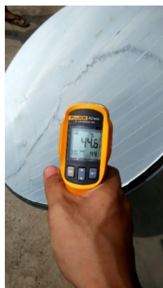
Figure-16: Temperature of concentrator measured using infrared thermometer (44.6 degree Celsius).
