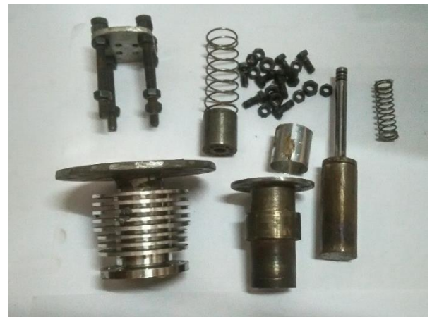
Figure-12: Parts before joining them with bolts and nuts.
