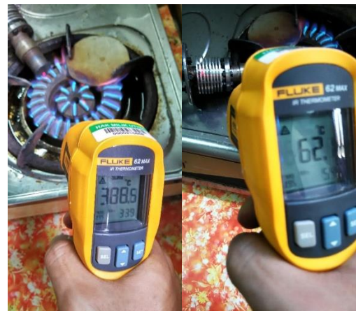
Figure-18: Temperature measured at heater end and cooler end.
