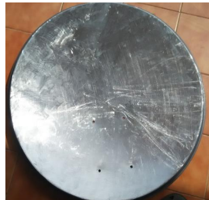
Figure-10: ASTRO satellite dish that has been sanded.
