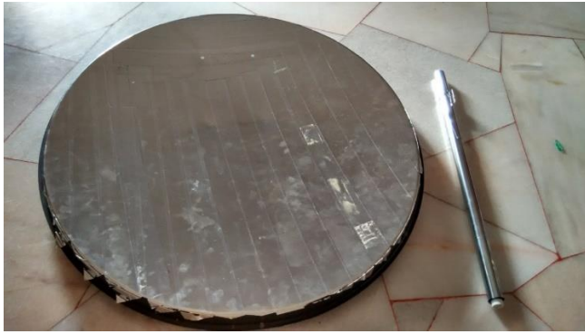
Figure-11: Parabolic dish concentrator made from Astro satellite dish by pasting the surface with solar reflective film.
